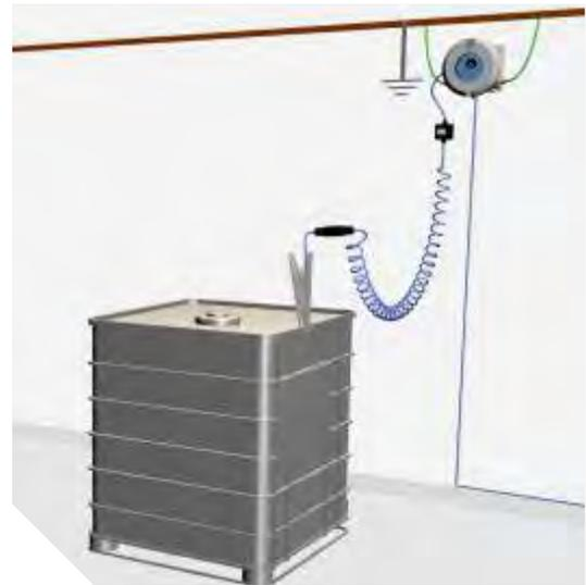
Conductive metal objects like tank cars, LACT units, skids and IBCs that come into contact with electrostatically charged liquids can accumulate hazardous levels of electrostatic charge that could discharge static sparks with energies far in excess of the minimum ignition energies of a vast range of combustible gases and vapors.
