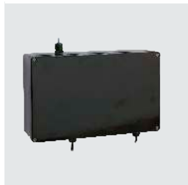
The Earth-Rite® MULTIPOINT II's 230 V/110 V AC power supply unit houses eleven (11) SP/DT volt free contacts. 8 of these interface with each monitored grounding channel, 2 provide the grouped channel function and 1 relay provides the fail-safe redundancy output function. The power supply can be installed in Zone 2/21 and Class 1, Div.2, Class II, Div.1, Class III, Div.1 areas. The power supply can be housed in GRP or stainless steel enclosures.
