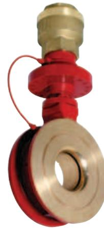
The SOLBERG Foam Pump Proportioner is manufactured using a bronze body and bronze pressure balancing valve for corrosion resistance. The SOLBERG Foam Pump Proportioner is to be installed with a minimum of 5 pipe diameters (30.0" (762 mm)) of straight pipe both upstream and downstream of the proportioner. The proportioner body is cast with a directional flow arrow on the proportioner body indicating the proper orientation of installation.
