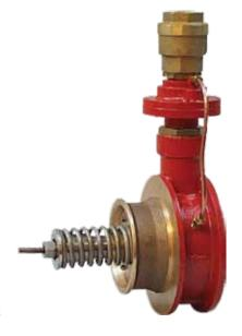
used as an integral component of a SOLBERG foam pump proportioning system. The SOLBERG Variable Range Pump Proportioner is designed to be installed as a between-the-flange proportioner, in standard 6.0" (152 mm) or 8.0" (203 mm) system piping. The foam concentrate inlet is 2.0" (50 mm) or 2.5" (64 mm) BSP female pipe size depending on the proportioner size selected.
